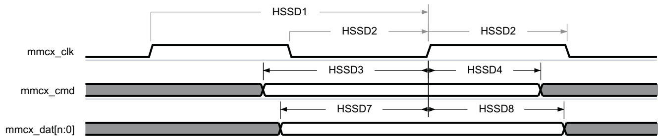
Figure 6-73. MMC2 and MMC3 Interfaces—High-Speed SDIO Mode—Data/Command Receive (1)
