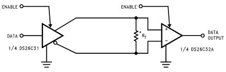
\*R<sub>T</sub> is optional although highly recommended to reduce reflection.
