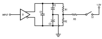
Note: C1 = C2 = C3 = 40 pF (Including Probe and Jig Capacitance), R1 = R2 =  $50\Omega$ , R3 =  $500\Omega$ .
