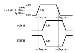
Figure 27. Propagation Delays
