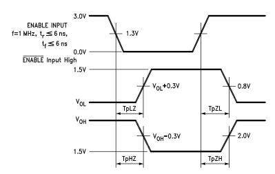
Figure 28. Enable and Disable Times
