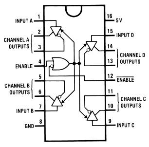
Figure 1. CDIP, CLGA Packages- Top View See Package Numbers NFE0016A, NAD0016A
