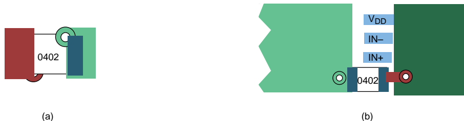
Figure 30. Typical Decoupling Capacitor Layouts
