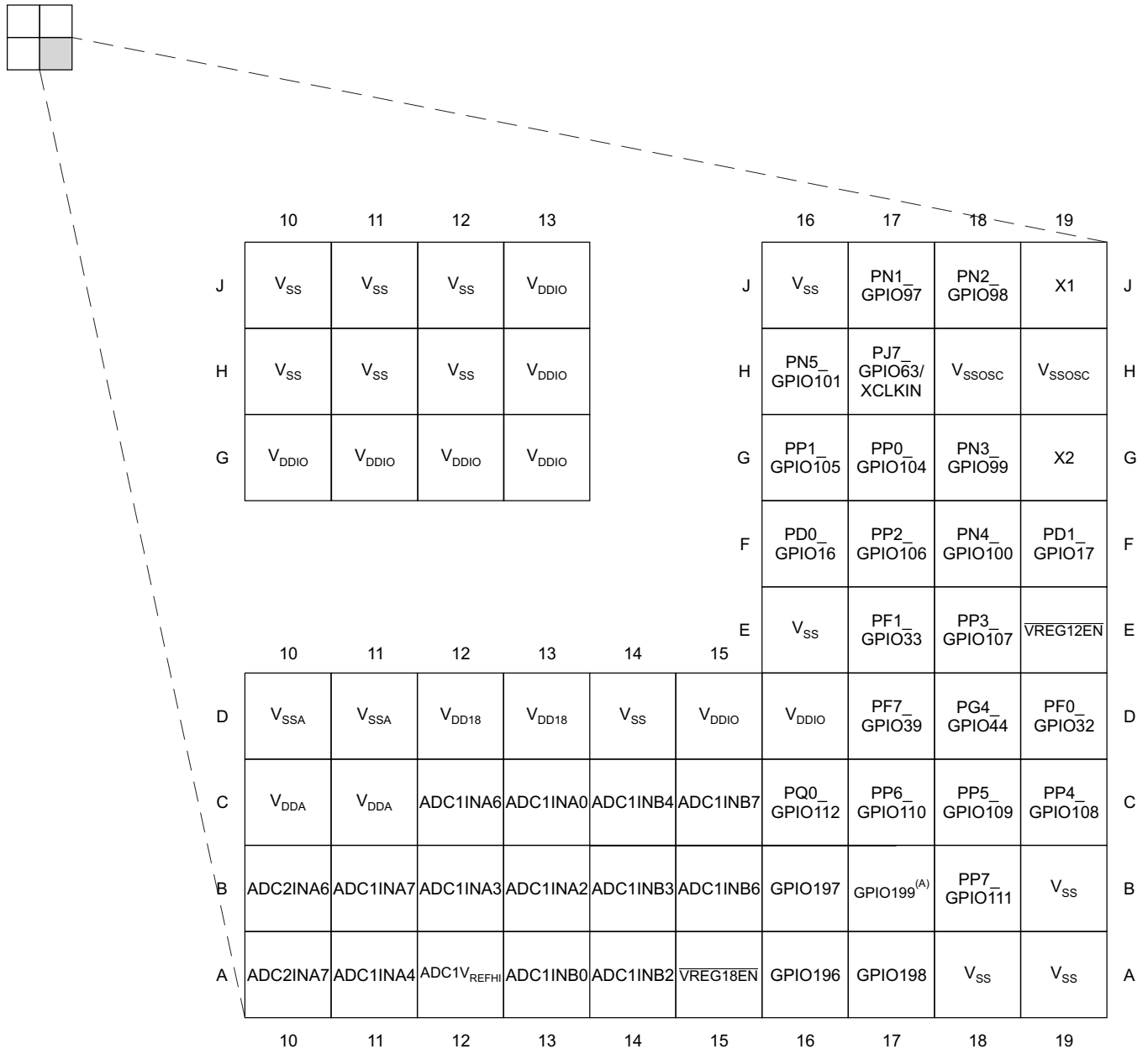
Figure 4-4. 289-Ball ZWT New Fine Pitch Ball Grid Array (Bottom View) – [Quadrant C]
