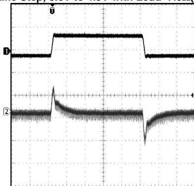
CH1: V_{IN} ; Scale: 1V/Div, AC Coupled CH2: V_{OUT} ; Scale: 20mV/Div, AC Coupled Time scale: 40 \mu s/Div
