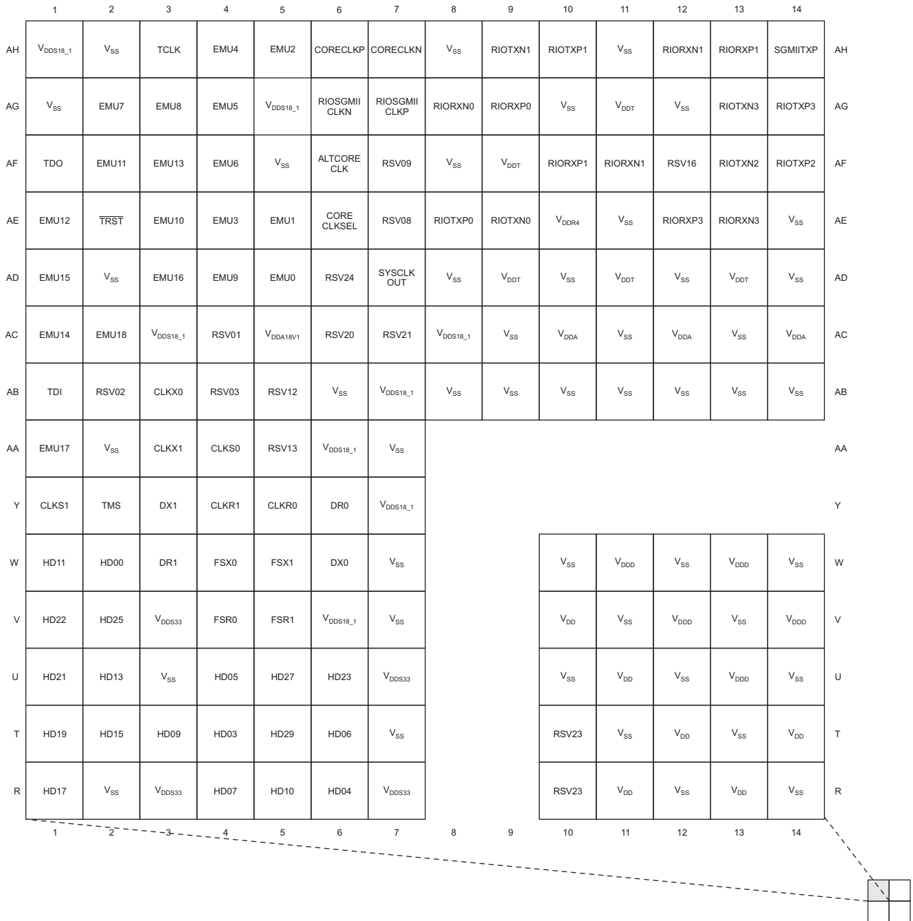
Figure 3-2. SM320C6457-HIREL Pin Map (Bottom View) [Quadrant A]
