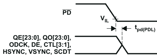
图 8-7. Delay From \overline{PD} Low to Hi-Z Outputs
