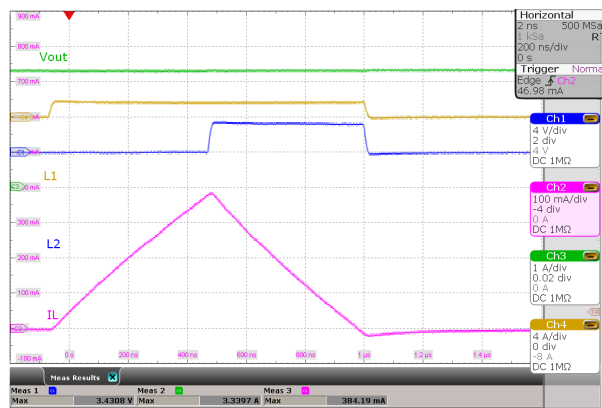
图 8-10. Switching Waveforms, Boost Operation
