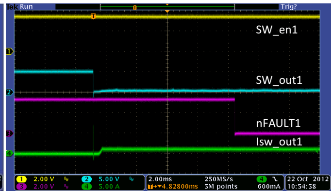
Figure 41. USB Switch1 Current Limit Operation
