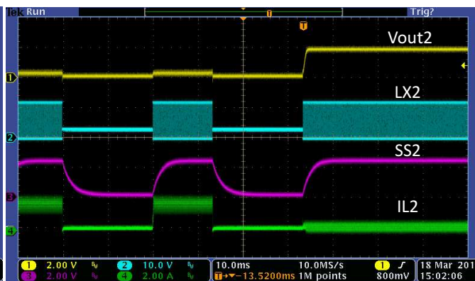
Figure 35. Hiccup Recover, Buck2=1.8V
