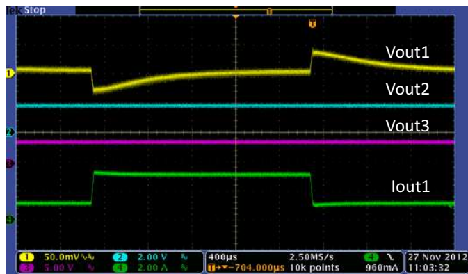
Figure 22. Transient Response Buck1@1.2V, 1-3A Step, C_o = 68\ \mu\text{F}
