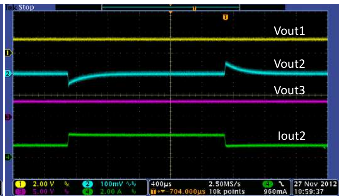
Figure 23. Transient Response Buck2@1.8V, 1-2A Step, C_o = 47\ \mu\text{F}
