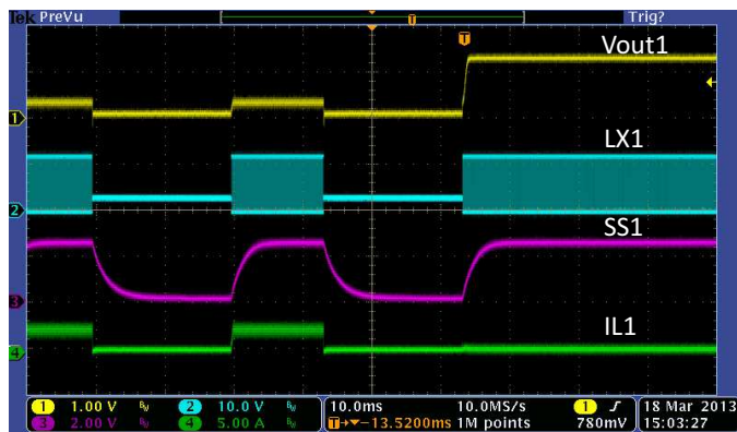
Figure 34. Hiccup Recover, Buck1=1.2V
