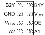
图 6-2. DTT Package, 8-Pin SON Transparent (Top View)
